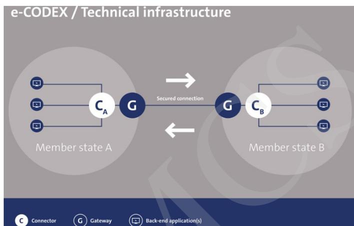
Figure 1. The technical architecture of the e-Codex system
